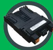
\* Support of real-time EtherNet (RTMoE), HTTP, SMTP, EtherNet/IP and Modbus TCP/IP
