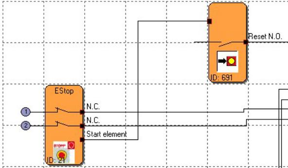
Correct connection between Reset element with use for monitored start up checked and the output connected to the Estop Start element input. The Estop has **Start behaviour monitored** checked.
