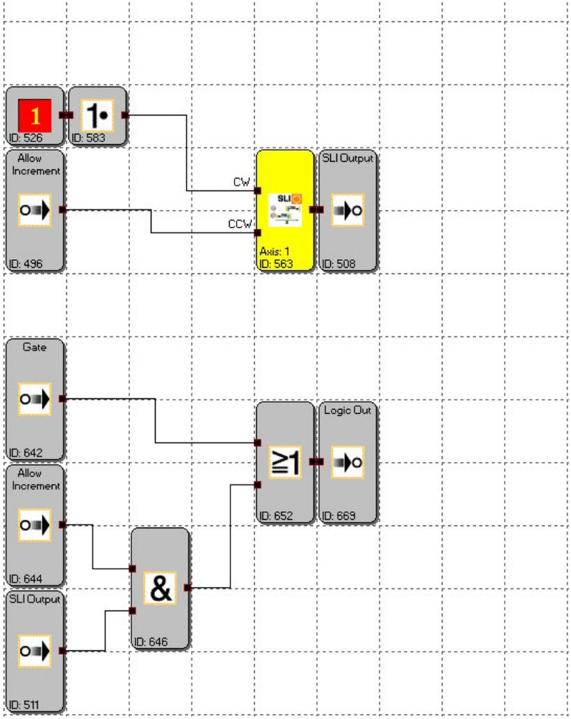
In this example Safe Gate Access (Gate OTE) is combined with Safe Limited Increment. In normal operation when the gate is opened (Gate In is FALSE) Logic Out will become FALSE which controls the STO and Brake Outputs.
