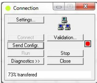
**NOTE** Cannot download to the SI-Safety if it is in an Error state. Must be in Stop State.
