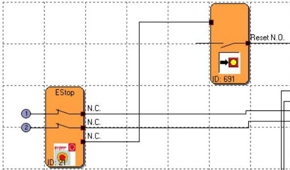
Error: The Estop has **Start behaviour auto** checked. The connection remains but the text has changed to N.C. The program can be compiled successfully.
