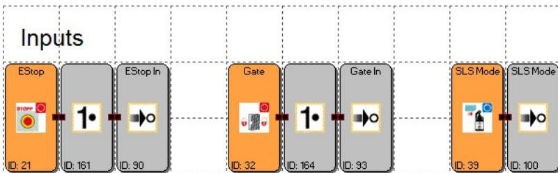
Each input is linked to an ITE (In Terminal Element). Depending on the logic requirements of downstream code it can be suitable to invert the input signal before linking to the ITE. Most safety devices are TRUE when in the safe state and FALSE when in the unsafe state. The safe monitoring functions are active when the input is TRUE. Thus to activate a safe monitoring function when the safety device is in the unsafe state (FALSE) the input will need to be inverted.
