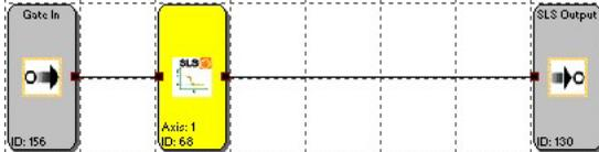
In this example SLS is used to implement a gate access safe limited speed function. The Gate In OTE is connected to the input of the SLS block. If the input is FALSE the block is not active. A rising edge at the input (input becomes TRUE) activates the block. The setup is as per the settings with all extended settings disabled. The output will remain TRUE unless the speed exceeds 30 rpm.
