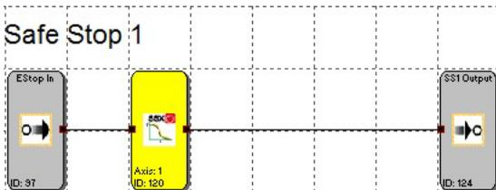
In this example SS1 is used to implement an E-Stop function. The Estop OTE is connected to the input of the SSX block. If the input is FALSE the block is not active. A rising edge at the input (input becomes TRUE) activates the block. The output will remain TRUE during the deceleration
