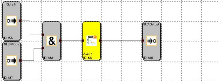
In this example Safe Stop 2 is combined with Safe Limited Speed. The SLS mode switch is used to switch between the two safety functions. When SLS Mode is TRUE, opening the gate (Gate IN is FALSE) will activate SLS. When SLS Mode is FALSE, opening the gate (Gate IN is FALSE), will activate the Safe Stop 2 safety function.
