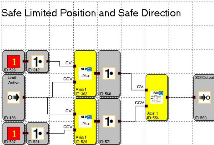
In this example Safety Limited Position is combined with Safe Direction to achieve end of travel limits but still allowing safe travel away from the limit.
