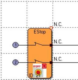
Error: The same as the above but the connection point has moved to the top right corner of the Estop block. When compiled the program will give the following error message:
